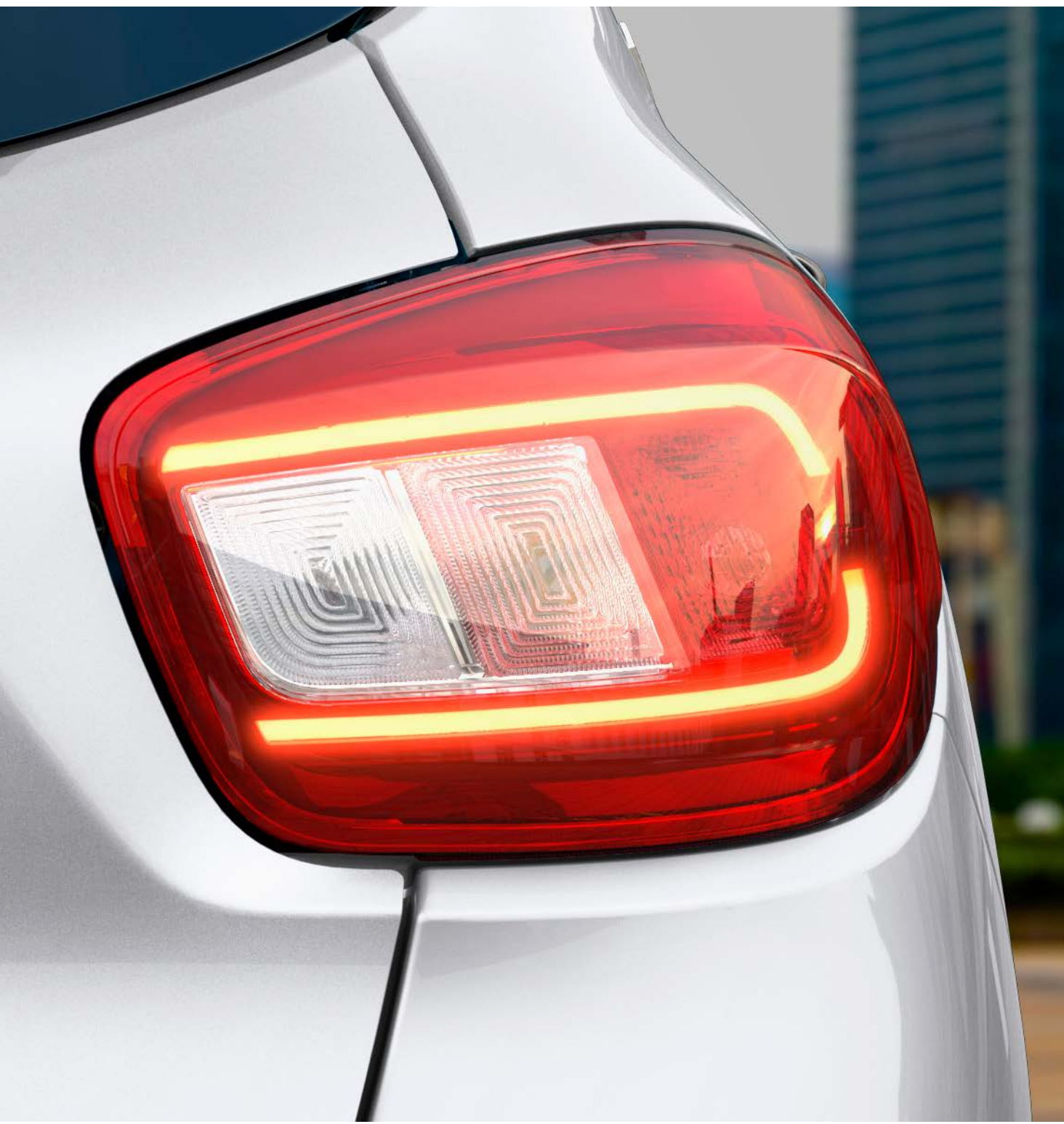
tail lamps with LED light guides
