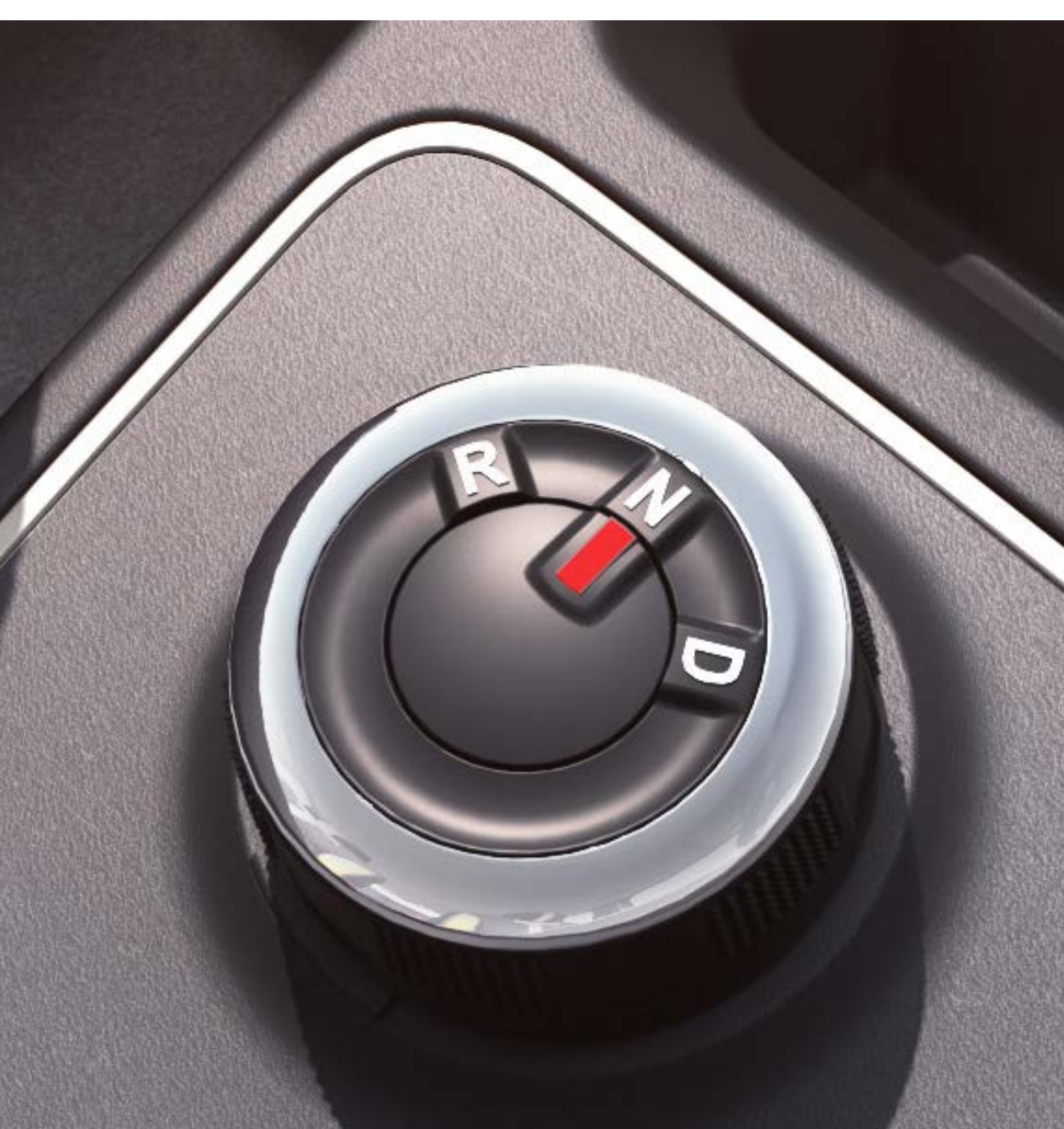
floor console mounted AMT dial
